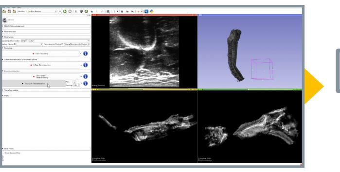
Full 3D intensity maps of the anterior surface of the arm were assembled from 2D ultrasound data (localized via motion capture) using an adapted version of the first OpenArm experimental protocol [5].
