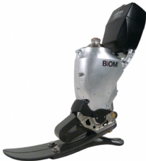
Figure 2: The BiOM active ankle-foot prosthesis.
